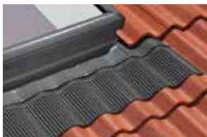
ECL – Shingles/shakes Step flashing pieces interweave with roofing material for proper water drainage. For use with shingles or shakes less than 3/4" thick.
